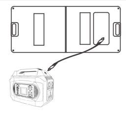
Do not place the charged device in direct sunlight or heated environment. Place the device in the pocket of the panel or in the shade while charging.
